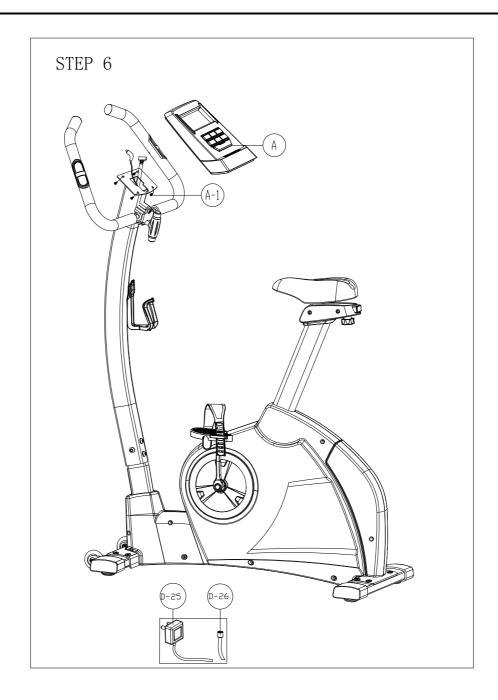
Connect the pulse cable coming out of the handlebar and the computer cable to the computer (A). Place the computer to the computer mast and fasten with Screws (A-1). Then the assembly is done.
