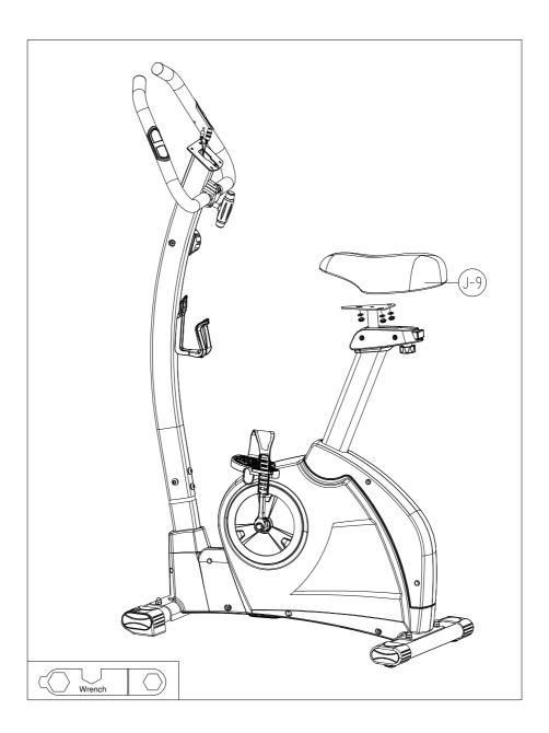
1. Fasten the saddle (J-9) to the seat post with screws.
