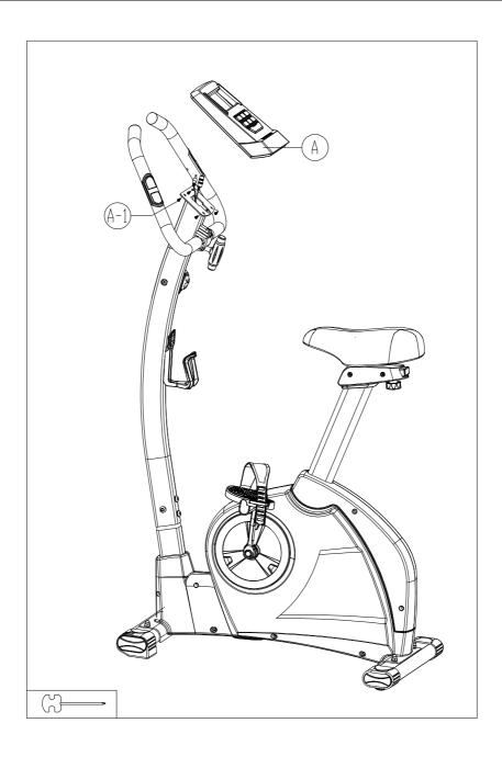
Connect the pulse cable coming out of the handlebar and the RPM sensor cable to the computer (A). Place the computer to the computer mast and fasten with Screws (A-1). Then the assembly is done.
