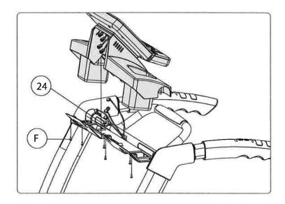
Note: Be careful to properly connect all wiring connectors with their correct corresponding wiring harness. Pay attention not to bend any pins and make sure the connectors click in place.
