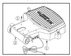
Fit the UPRIGHT TUBE - LOWER [002] over the exposed bolts and fit 4 x WASHERS [400] and 4 x NUT [200]. Tighten very firmly.
