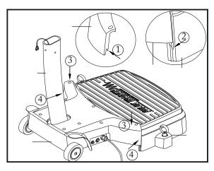
For packing purposes only, the HANDLE BAR [005] was bolted to the UPRIGHT TUBE-UPPER [003]. Remove x 2 BOLT [301] and continue the assembly process.
