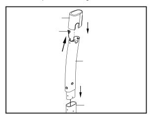
Secure the HANDLE BAR [005] with 2 x BOLT [301], 8 x BOLT [300] with 4 x WASHER [406] (curved) and 4 x WASHER [407]. Side the UPRIGHT TUBE COVER [110] over the bottom section of the HANDLE BAR. Push firmly. It was designed to be a tight fit.
