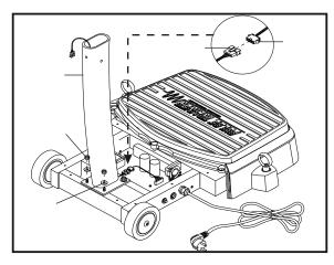
Slide the REAR COVER [100] over the UPRIGHT TUBE-LOWER [002] and COMPUTER CABLE [704].
