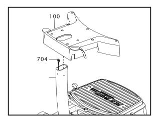
Carefully slide the REAR COVER [100] onto the FRONT COVER [101] observing the mating ribs. NOTE: Make sure the REAR COVER is kept level during the alignment and fitting process. The covers are a good fit with each other. Do not fit SCREWS until STEP 10.
